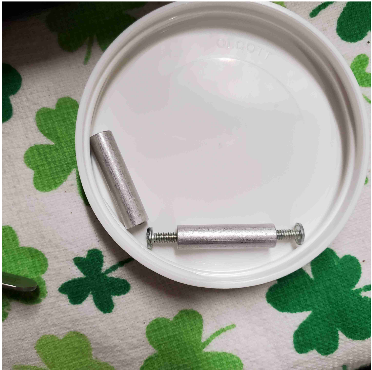
DOWELS THREADED FOR 4-40 SCREWS – ALL THE WAY THROUGH
