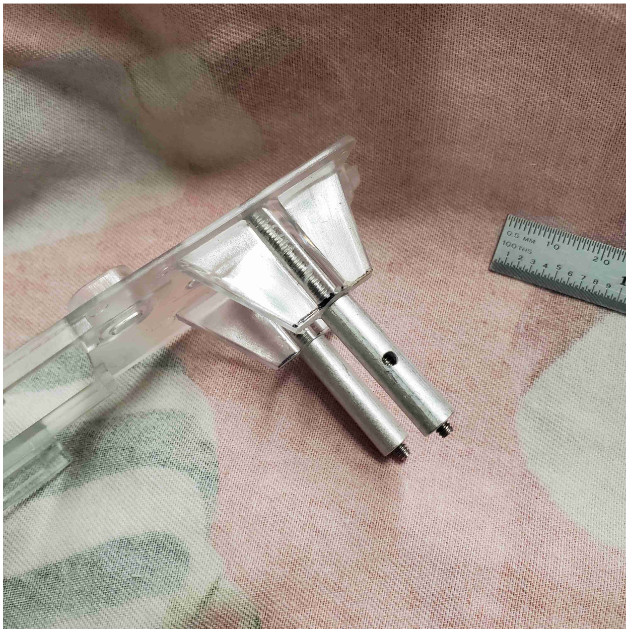
REAR DOWELS INSTALLED FOR FIT (SCREWS WILL BE CUT SHORTER FOR 2-56 TO SLIDE THROUGH)
