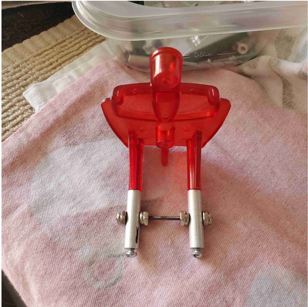
ANTI-TWIST 2-56 ALL THREAD WITH LOCKING NUTS ALSO MAINTAINS POST SPACING (POSTS ARE REALLY PARALLEL – PIC MAKES THEM LOOK SPREAD)
