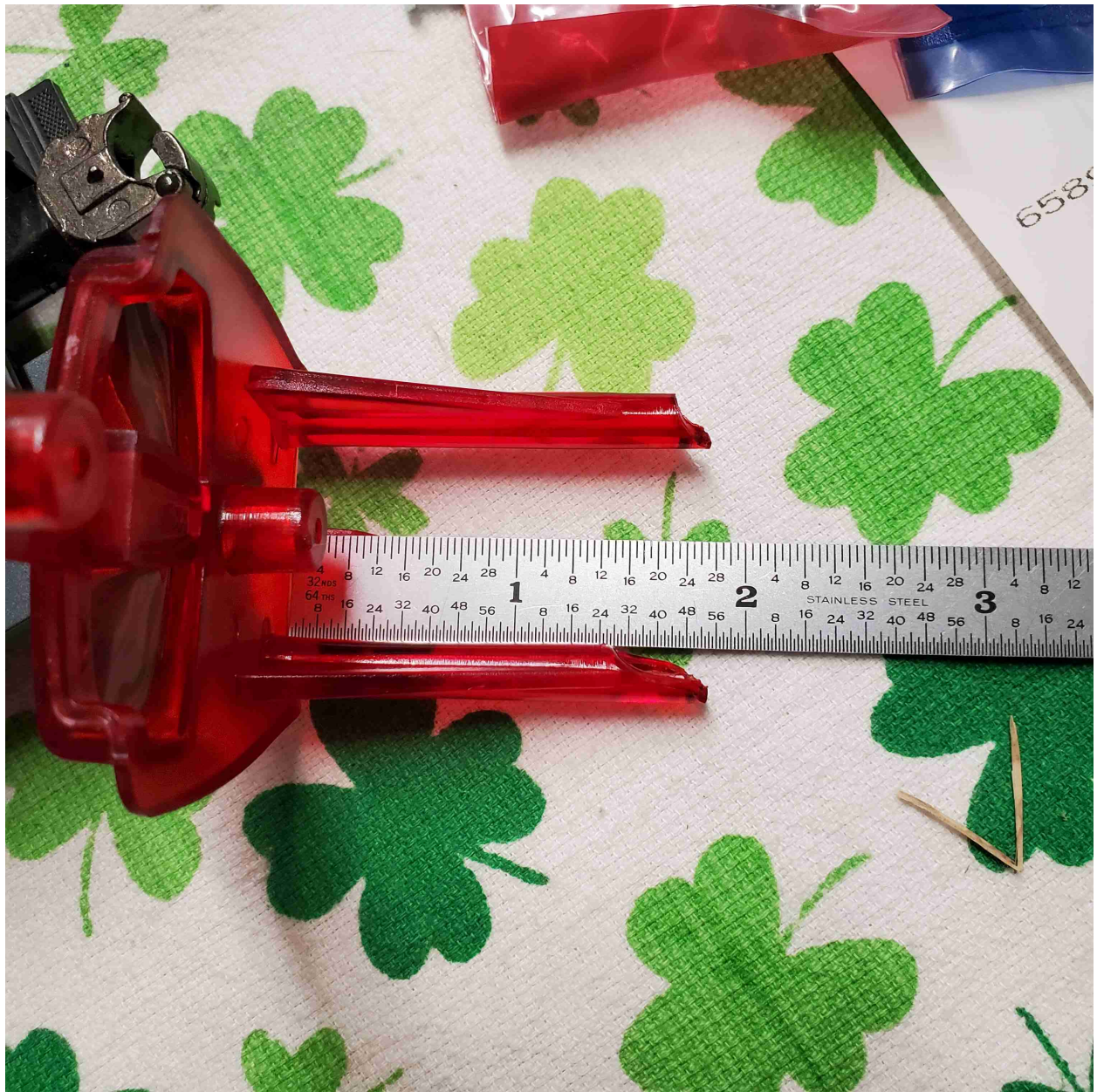
MEASURING FOR FRONT DOWELS PLASTIC TO BE CUT OFF WITH DREMEL TOOL
